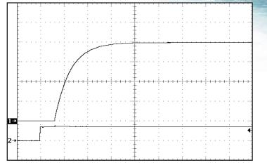
Figure 8: Turn-on transient at full resistive load and 3mF output capacitance initiated by ENA1. Input voltage pre-applied. Ch 1: Vout (3V/div). Ch 2: ENA1 (5V/div). Horizontal Timescale: 5msec/div.
