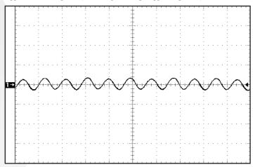
Figure 16: Output voltage ripple, Vout, at nominal input voltage and rated load current (20mV/div). Load capacitance:  $1\mu F$  ceramic capacitor and  $10\mu F$  tantalum capacitor. Horizontal Timescale:  $2\mu sec/div$ . Bandwidth: 10MHz. See Figure 14.
