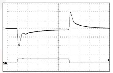
Figure 12: Output voltage response to step-change in load current 0%-50%-0% of lout (max). Load cap:  $1\mu$ F ceramic cap and  $10\mu$ F,  $100m\Omega$  ESR tantalum cap. Ch 1: Vout (200mV/div). Ch 2: lout (10A/div). Horizontal Timescale: 100µsec/div.
