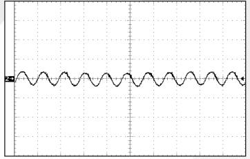
Figure 15: Input terminal current ripple, ic, at full rated output current and nominal input voltage with SynQor MQ filter module (50mA/div). Horizontal Timescale: 2µsec/div. Bandwidth: 20MHz. See Figure 14.
