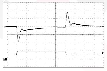
Figure 11: Output voltage response to step-change in load current 50%-100%-50% of Iout (max). Load cap:  $1\mu$ F ceramic cap and  $10\mu$ F,  $100m\Omega$  ESR tantalum cap. Ch 1: Vout (200mV/div). Ch 2: Iout (10A/div). Horizontal Timescale: 100µsec/div.
