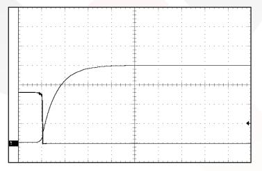
Figure 17: Rise of output voltage after the removal of a short circuit across the output terminals. Ch 1: Vout (3V/div). Ch 2: Iout (5A/div). Horizontal Timescale: 5msec/div.
