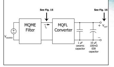
Figure 14: Test set-up diagram showing measurement points for Input Terminal Ripple Current (Figure 15) and Output Voltage Ripple (Figure 16).
